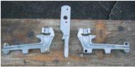
The T.Mclachlin no 18 molds and plunger – note there is no vent on the mold beneath the bowl.
